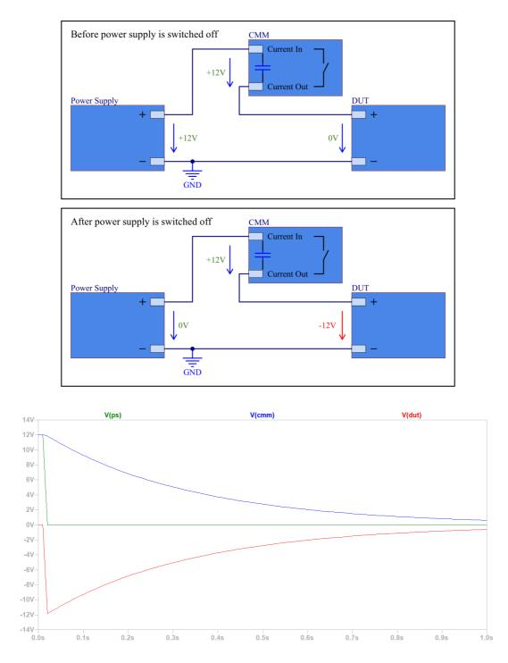
This problem mainly occurs with DUTs which have a high input impedance (for example a DUT in sleep mode) and therefore cannot discharge the capacitor quickly. The negative voltage could either damage the DUT or a connected measurement device like the MesSy-II.
