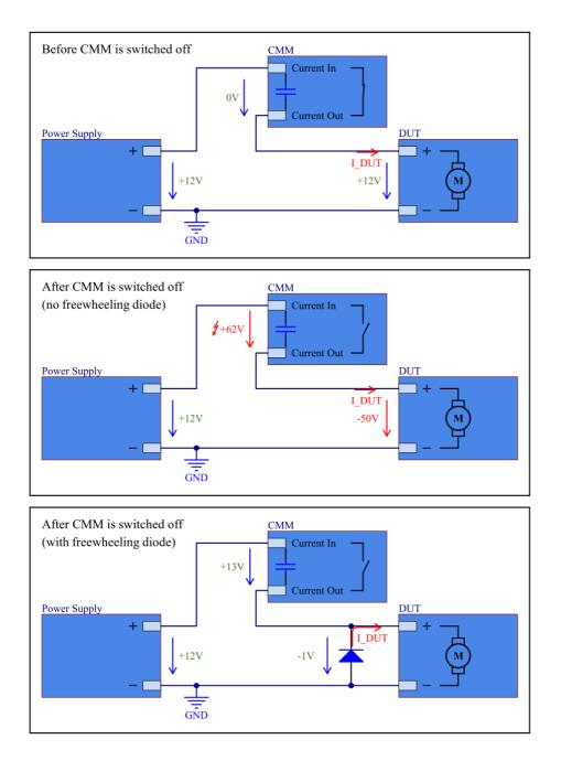
If you need to switch the CMM while an inductive load is connected, you must always connect a freewheeling diode to the load to protect the CMM. Our recommendation is NOT to use the CMM as a load switch. Use a suitable load switch instead.
