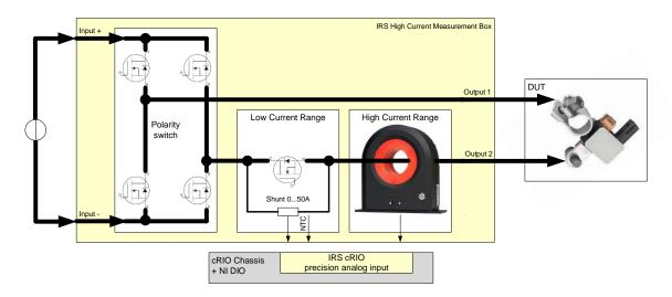
An external standard power supply feeds the energy into the HCMB. Via the integrated polarity switch either positive or negative current may be selected. The current passes the two measurement stages for currents below and above 50A and is finally output to the DUT. Please note that the power supply only has to provide enough voltage for covering the voltage drops on DUT and HCMB.
